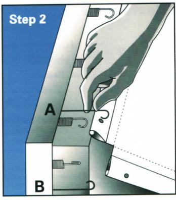
**Step 2.**Hook the face on to the Prespacers located in the sign box at A - B - C - E - F
