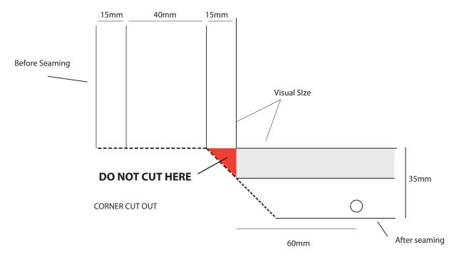
Punch Holes 60mm from each end. Up to 2999mm in Height 150mm Hole Centres all round 3000mm and above in Height 100mm Hole Centres all round
